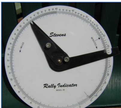
The Stevens rally wheel is a circular slide rule that was commonly used in rallies in the 1960s and 70s.
